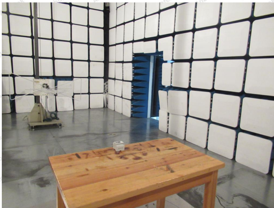
Photo of Radiated Emission Test
