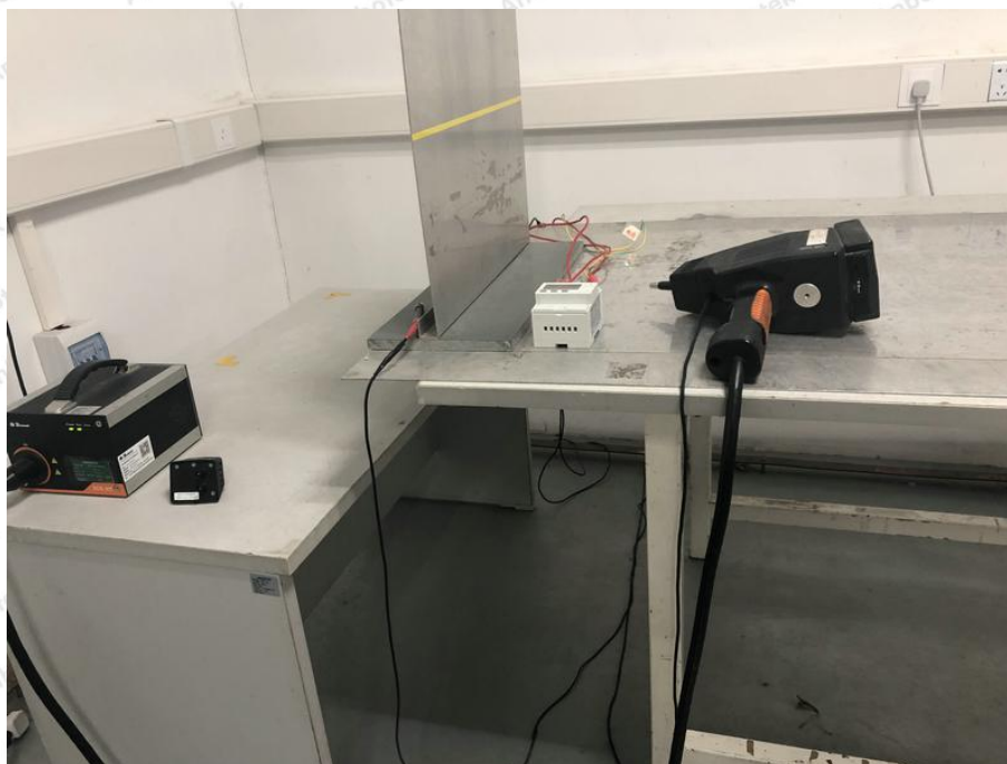
Photo of Electrostatic Discharge Immunity Test
