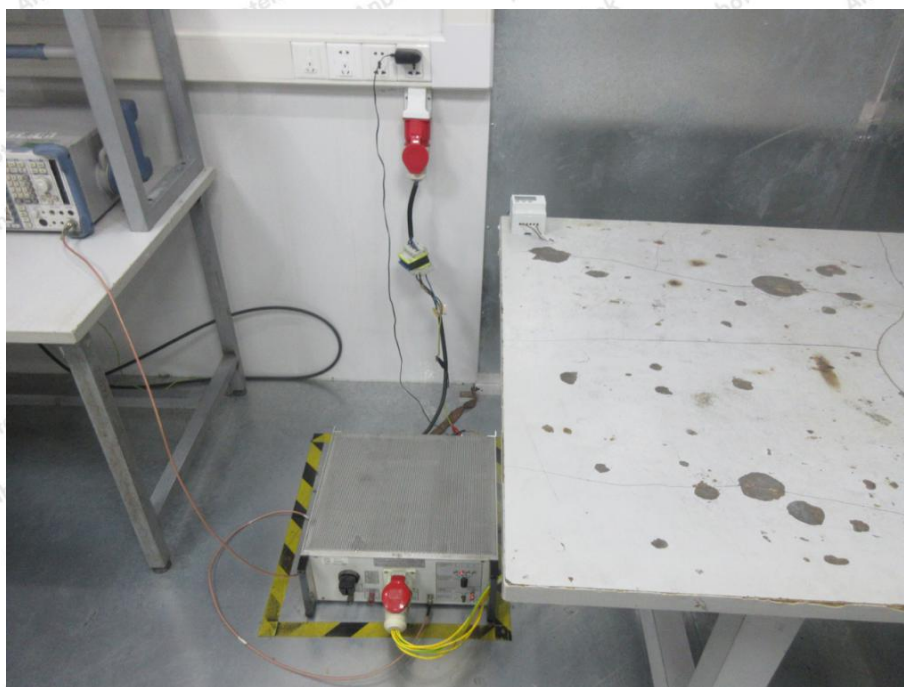
Photo of Power Line Conducted Emission Test
